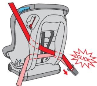
**Step 2:** Pull out the vehicle's seat belt (diagonal and lap belt) and insert it through the belt loop in the backrest. Clip in the seat belt buckle. A "click" will indicate that it is attached correctly.
