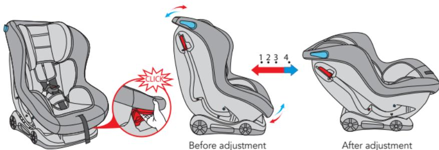
The car seat can be placed in 4 different inclination positions.
