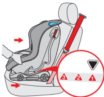
**Step 1:** Adjust the car seat in the desired position: 1, 2 or 3.
