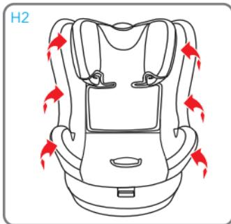
Remove it, carefully pulling the fabric off from the frame, starting from one side, being careful while removing the fabric from the lap belt guide.
