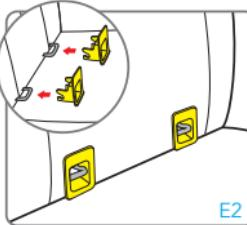
Locate the ISOFIX attachments supplied with the vehicle (E2). If your car does not have standard ISOFIX connector guides, insert those supplied with the car seat with the recess facing upwards in the two ISOFIX anchoring points in the car.
