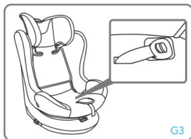
Lift up the seat lining and remove the crotch belt from its housing compartment.
