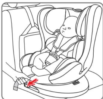
**Tightening the harness:** Pull the harness adjustment strap so as to tighten it properly against the body of the child. The harness is correctly tightened when the gap between the harness and the child is no greater than the thickness of your finger (1 cm).
