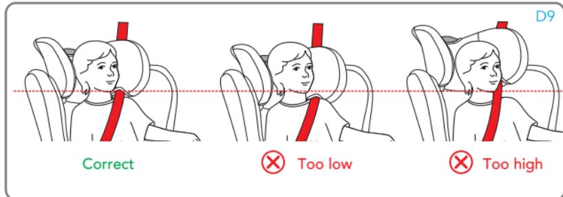
When using the 3-point vehicle seat belt, the headrest must be adjusted so that there is a two-finger space between the headrest and the child's shoulders. Make sure that the diagonal belt, when passing through the "diagonal belt guide loop" on the side of the headrest, is positioned at the shoulders and not at the child's neck.
