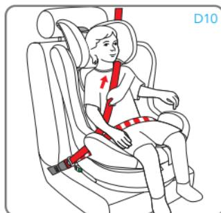
D10 Tighten the belt as shown in the figure.
