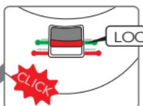
Rotate the seat into the rear-facing position, a "click" will indicate that it is locked.
