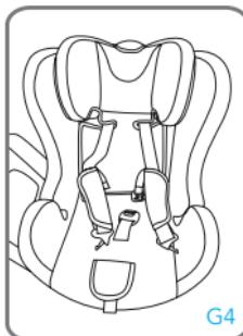
Replace the fabric on the backrest and seat. Thread the buckle with crotch strap through the slot on the seat. Thread the chest protector straps through the slots in the backrest fabric and through the slots in the shell.
