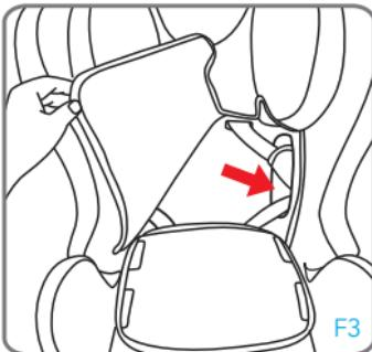
Lift up the fabric lining from the backrest and insert the chest belt with the respective ends into the specific left side and right side compartment.
