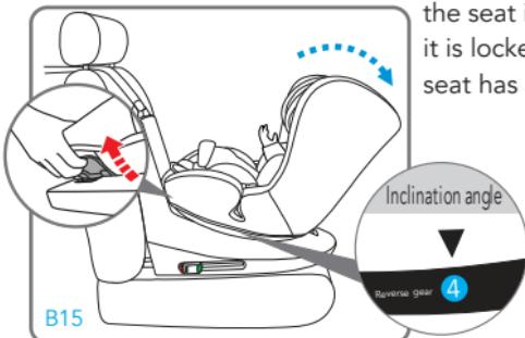
**CAUTION!** The car seat can only be reclined in the most horizontal inclination (4) when it is installed in the rear-facing position. The use of other inclinations is not allowed.
