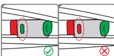
Align the ISOFIX connectors with the anchoring points fixed to the vehicle passenger seat and press until you hear a "click". The indicator on both brackets will turn green, confirming that they have attached. Ensure that both brackets are correctly fastened. Shake the car seat to be sure it is correctly fixed in place.
