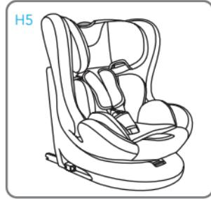
Make sure that it has been assembled correctly, checking that the harness belts are not twisted
