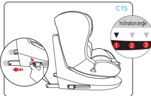
Press the adjustment handle located under the front of the car seat and, holding it down, pull or push the seat forwards or backwards. Release the handle when the seat is in the desired position and make sure that it is locked correctly; you will hear a "click" when the seat has attached.
