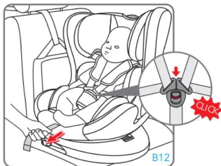
Place the child into the car seat. Place the straps over the child's shoulders, join together the two belt tabs and hook them to the buckle.
