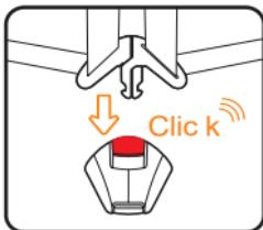
**To attach the buckle:** Hold together the central buckle tabs and insert them in the special slot inside the harness buckle. A "click" will indicate that it has attached correctly.
