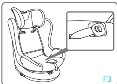
Lift up the seat lining and place the buckle in the compartment on the left side.
