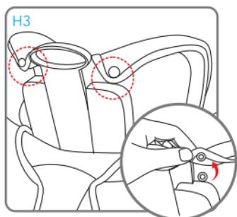
Place the seat lining on the car seat and insert the leg separator harness with protection into the slot.
