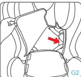
Lift up the fabric lining from the backrest. Remove the chest belts from the right and left compartment. Replace the fabric on the backrest.
