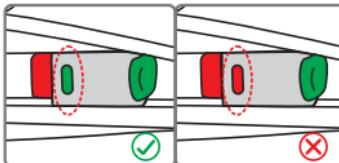
Align the ISOFIX connectors with the anchoring points fixed to the vehicle passenger seat and press until you hear a "click". The indicator on both brackets will turn green, confirming that they have attached. Ensure that both brackets are correctly fastened. Shake the car seat to be sure it is correctly fixed in place.
