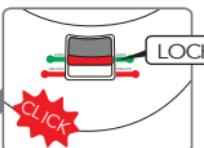
Rotate the seat into the facing position, a "click" will indicate that it is locked.
