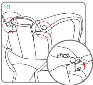
Loosen the harness and remove the reducer if it is being used.
