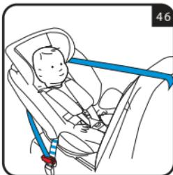
Shake the car seat to be sure it is firmly fixed in place (fig. 45).
