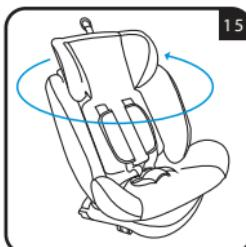
Press the rotation button and turn the seat of the car seat in the desired direction (fig. 14 and fig. 15).
