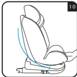
Press the adjustment handle located under the front of the car seat and, holding it down, pull or push the seat forwards or backwards. Release the handle when the seat is in the desired position and make sure that it is locked correctly; you will hear a "click" when the seat has attached (fig. 10).
