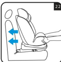
22 that the ISOFIX connectors are attached on both sides.
