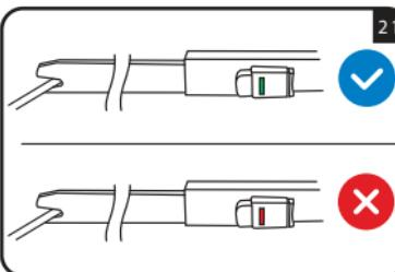
Insert the two ISOFIX connectors in the appropriate guides: a "click" will indicate that they have been inserted and
