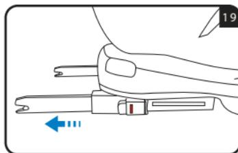
Press the ISOFIX buttons located on both sides of the seat and extend the ISOFIX connectors as much as possible (fig. 18 and 19).
