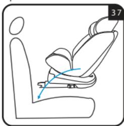
into the most horizontal position (see par. 4.4). Place the car seat so that it is in the rear-facing position (fig. 35, 36 and 37). **Use the reducer with children weighing less than 9 kg.**
