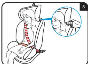
When using the 3-point vehicle seat belt, the headrest must be adjusted so that there is a two-finger space between the headrest and the child's shoulders. Make sure that the diagonal belt, when passing through the "diagonal belt guide loop" on the side of the headrest, is positioned at the shoulders and not at the child's neck (fig. 8).
