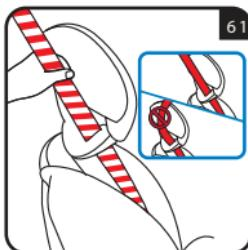
Insert the diagonal belt into the belt guide loop, making sure it is not twisted (fig. 61).
