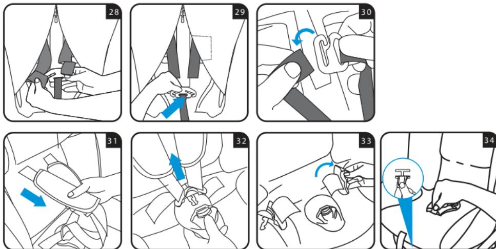
Unhook the chest belt straps from the belt tensioning bracket on the back of the car seat (fig.28)
