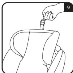
**To raise the headrest:** pull the headrest adjustment strap upwards.
