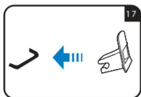
If your car does not have standard ISOFIX connector guides, insert those supplied with the car seat with the recess facing upwards in the two ISOFIX anchoring points in the car.
