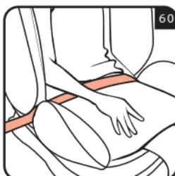
Thread the lap belt on the opposite side of the car seat into the lap belt loop (fig. 60).
